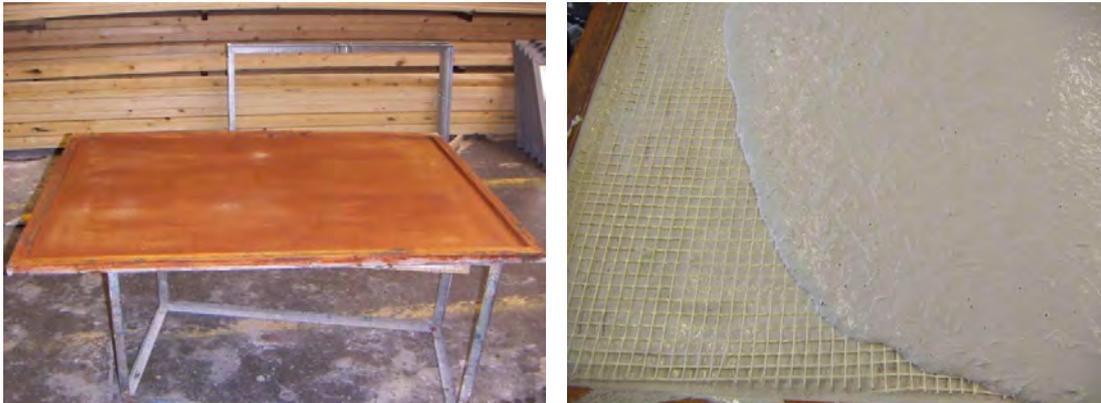
Figure 4 Mould and test board casting
