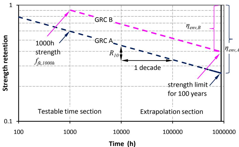
Figure 14 Environmental strength retention factor and 1000 h strength for two different GRC materials with different durability (adopted from fib bulletin 40)
