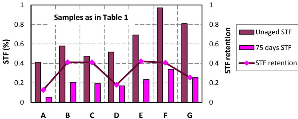
Figure 7 Residue STF after 75 days accelerated ageing
