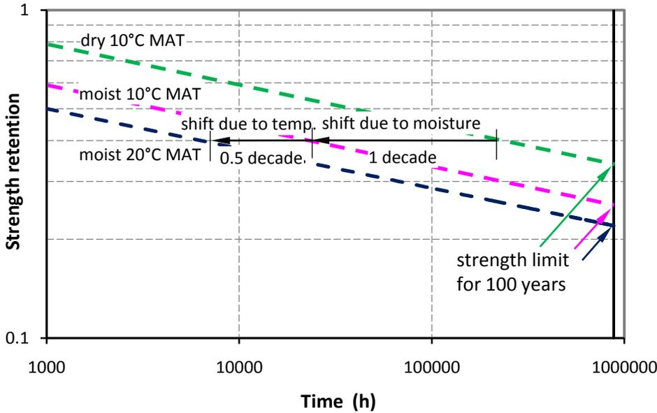
**Figure 15 Effect of the parameter of temperature and humidity on GRC flexural strength retention curves (adopted from Weber (2006))**
