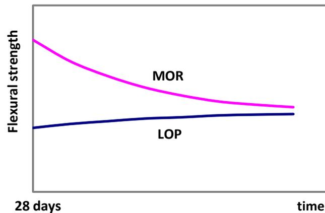
**Figure 1 Long term flexural strength declining**
