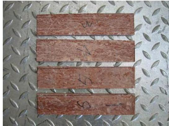
Figure 12 Bending test coupons
